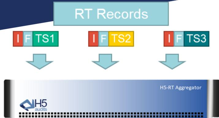
To consolidate the performance data provided by RT Agents, the H5-RT architecture includes an aggregation layer element: the RT aggregator.
