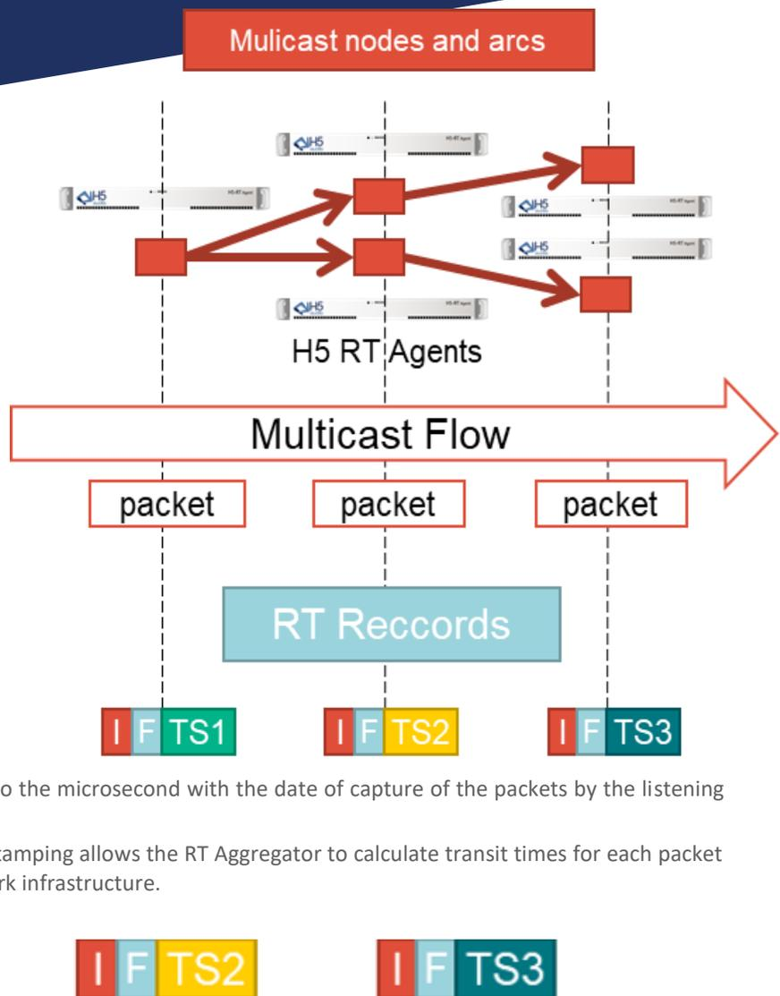
The RT records are grouped by the RT Agents in 1-minute intervals, compressed and made available to the RT Aggregator for download and processing.
